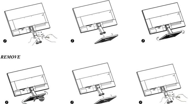
Figure.1. Installing and Removing the Base
