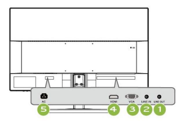
Figure.2. Connecting to a PC
